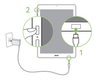
Plug in before turning on for the first time.
